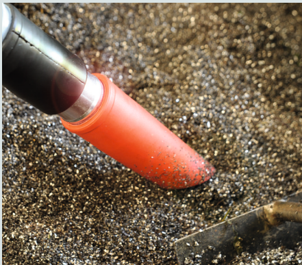
Recovery of metal chips
